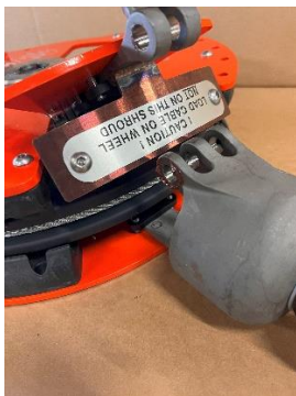
Properly loaded Line Figure 10
