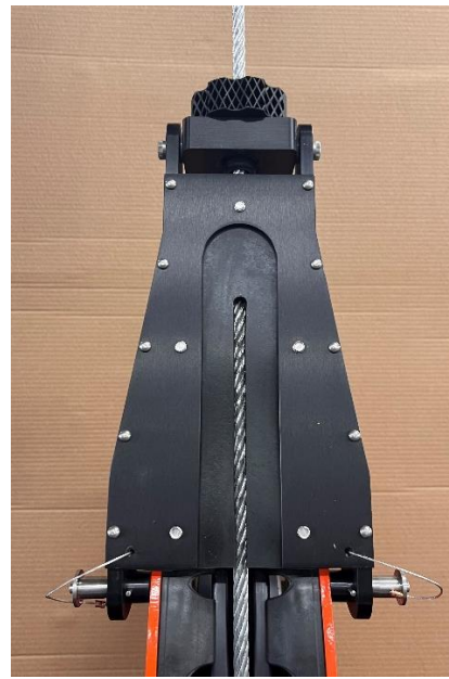
Properly Installed Quick Release Pin Figure 23
